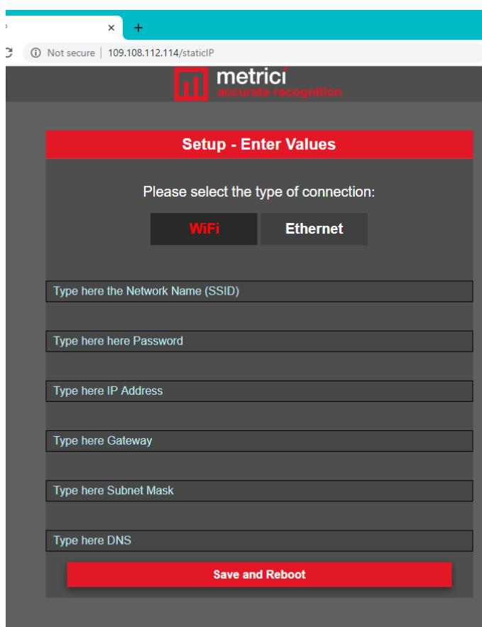
The WiFi setup interface shows a red header bar with the title "Setup - Enter Values". Below it, a message asks to select the type of connection, with "WiFi" highlighted in red. The form contains fields for Network Name (SSID), Password, IP Address, Gateway, Subnet Mask, and DNS. A red "Save and Reboot" button is at the bottom.
