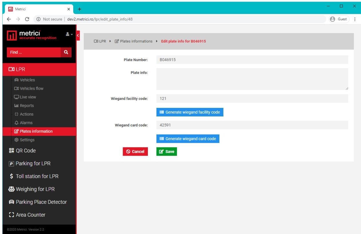
The screenshot shows the 'Edit plate info for B046915' dialog box. It contains fields for Plate Number (B046915), Plate info (empty), Wiegand facility code (121), and Wiegand card code (42591). There are also buttons for generating new codes ('Generate wiegand facility code' and 'Generate wiegand card code') and buttons for Cancel and Save.
