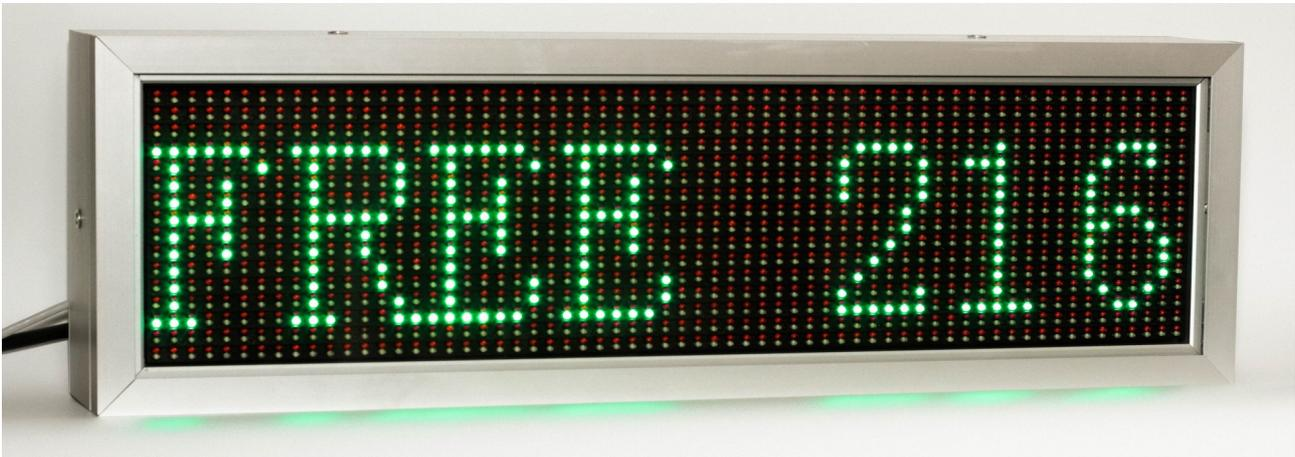
On a single row display (RG8x1, RG12x1, RG16x1) the information about Free and Busy spaces will alternate on screen. On a 2 rows display, these data will appear together on display.
