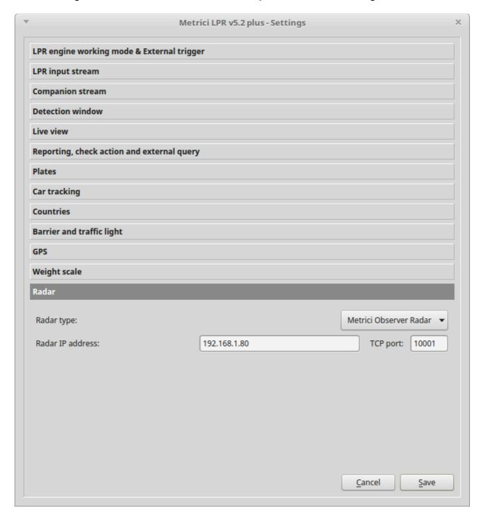
Choose the Radar Type, fill in its IP address (the default one is 192.168.1.80) and the TCP port as it is in the Barix Serial Settings.
