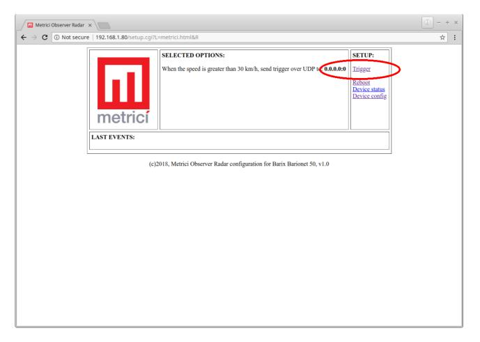
You will enter Metrici Observer Radar interface and the text "When the speed is greater than 30 km/h send trigger over UDP to 0.0.0.0". Choose **Setup, Trigge**r option to fill in the IP address.
